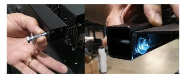
Step 4 Install and tighten the included nuts, and secure the stand to the charger. *If using power tools, wear proper eye protection and any other employer required PPE!*
