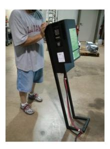
Step 6 Using the holes in the bottom portion of the stand, secure the charger stand to the mounting surface. Please note that mounting hardware is <u>not</u> included. *Caution! – The charge stand is top heavy, do not leave or use the charger unsecured in an upright position!*
